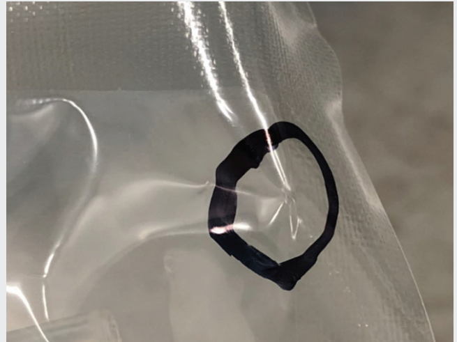
Closeup view, example of pinholes in corner of bags
